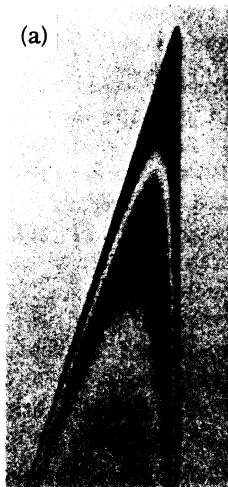
FIG. 7. Umweganregung pattern at (222) position in silicon; (a) using \text{CuK}\alpha_1 radiation, (b) using \text{AgK}\alpha_1 radiation. The zero of the azimuth was chosen with a [110] axis lying on both the (222) lattice plane and the diffraction plane. The positions in azimuth used are shown by the arrows.
