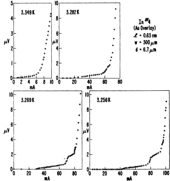
FIG. 2. Voltage vs current for an In microstrip at different temperatures (sample In-4).
