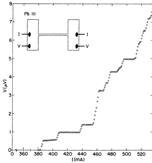
FIG. 1. Voltage vs current in a Pb microstrip at 4.2 K at the onset of the current-induced resistive state (sample Pb-111).
