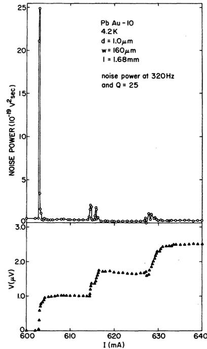
FIG. 4. Voltage and electrical noise power vs current in a Pb strip at 4.2 K (sample PbAu-10).
