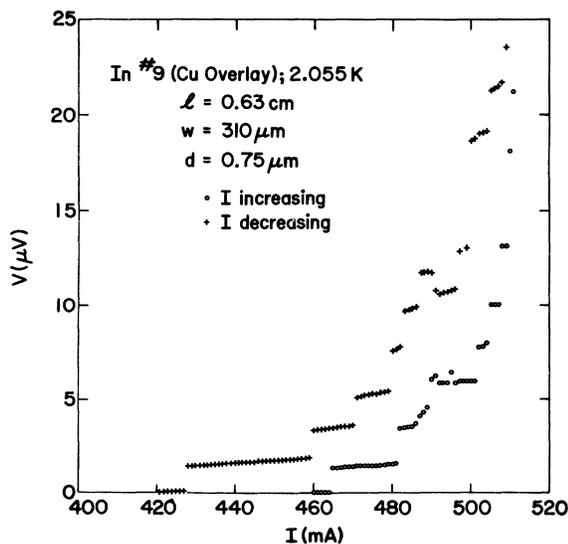
FIG. 3. Voltage vs current for an In strip at 2.055 K at increasing and decreasing current (sample In-9).
