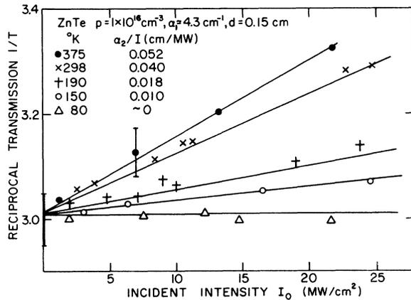
FIG. 5. Reciprocal transmission versus intensity of incident radiation for ZnTe measured at various sample temperatures.
