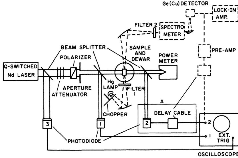
FIG. 3. Experimental arrangement with the Nd-glass laser alone is shown by solid lines. In the measurements using an additional light source, the part enclosed in A is replaced by the part shown by dashed lines.
