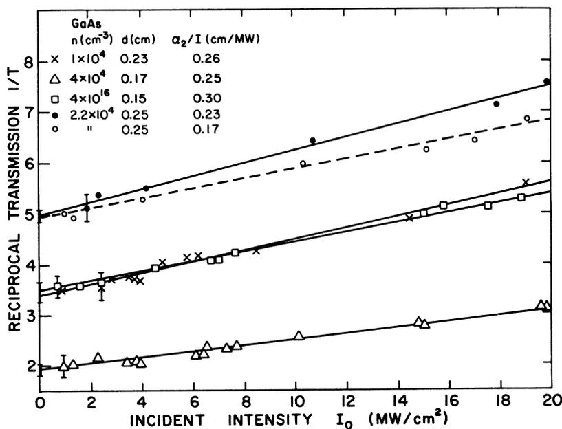
FIG. 8. Reciprocal transmission vs intensity of incident radiation for various GaAs samples. Solid lines are for RT. Dashed line is for  $\sim 15^\circ\text{K}$ .
