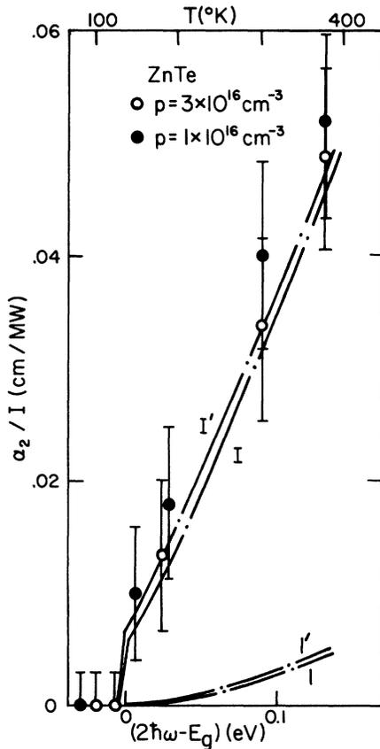
FIG. 6.  $\alpha_2/I$  deduced from measurements for the ZnTe sample (open circles for  $P=3 \times 10^{16} \text{ cm}^{-3}$ , closed circles for  $p=1 \times 10^{16} \text{ cm}^{-3}$ ). Curves I and 1 are calculated theoretically with and without exciton effect. Curves I' and 1' are calculated correspondingly with an additional band  $\Gamma_7$ .
