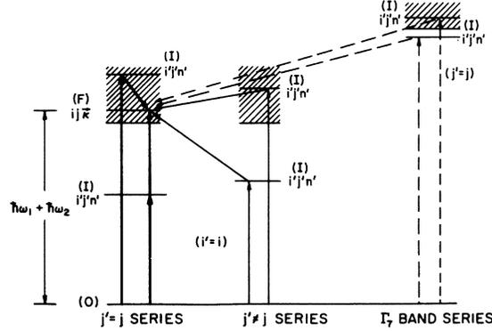
FIG. 2. Two-photon transition processes in the presence of exciton effect. The ground state is denoted by 0, the intermediate states are denoted by  $I$  or  $i'j'n'$ , the final states are denoted by  $F$  or  $ij\vec{k}$ . Transitions within one exciton series and transitions involving two different series are shown by heavy and thin arrows, respectively. Transitions involving the extra band  $\Gamma_7$  are shown by dashed arrows.
