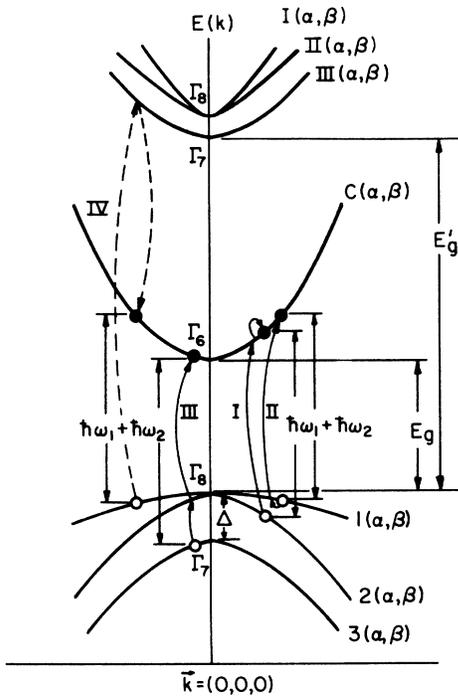
FIG. 1. Schematic diagram of two-photon transition processes. Type-I process involves an intra-conduction-band transition, type-II process involves an intra-valence-band transition, and type III involves an inter-valence-band transition. Type-IV process involves another energy band.
