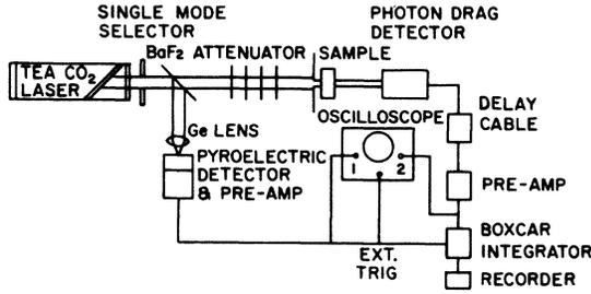
FIG. 4. Experimental setup with the CO<sub>2</sub> laser.
