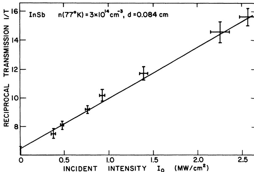
FIG. 7. Reciprocal transmission vs intensity of incident radiation for InSb measured at RT.
