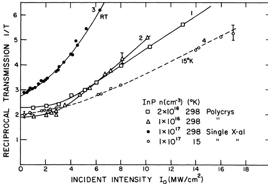
FIG. 10. Reciprocal transmission vs intensity of incident radiation for various InP samples. Solid lines are for RT. Dashed line is for  $\sim 15^\circ\text{K}$ .
