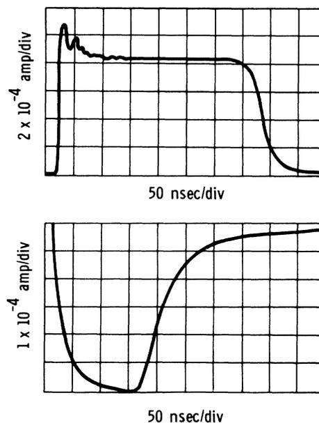
FIG. 1. Current vs time as observed in a  $190\text{-}\mu\text{m}$ -thick crystal with  $2500 \text{ V}$  applied. These figures were traced from oscilloscope pictures. The top picture was obtained by irradiating the negative electrode, so electrons are traversing the crystal and the bottom picture was obtained by irradiating the positive electrode, so holes are traversing the crystal.
