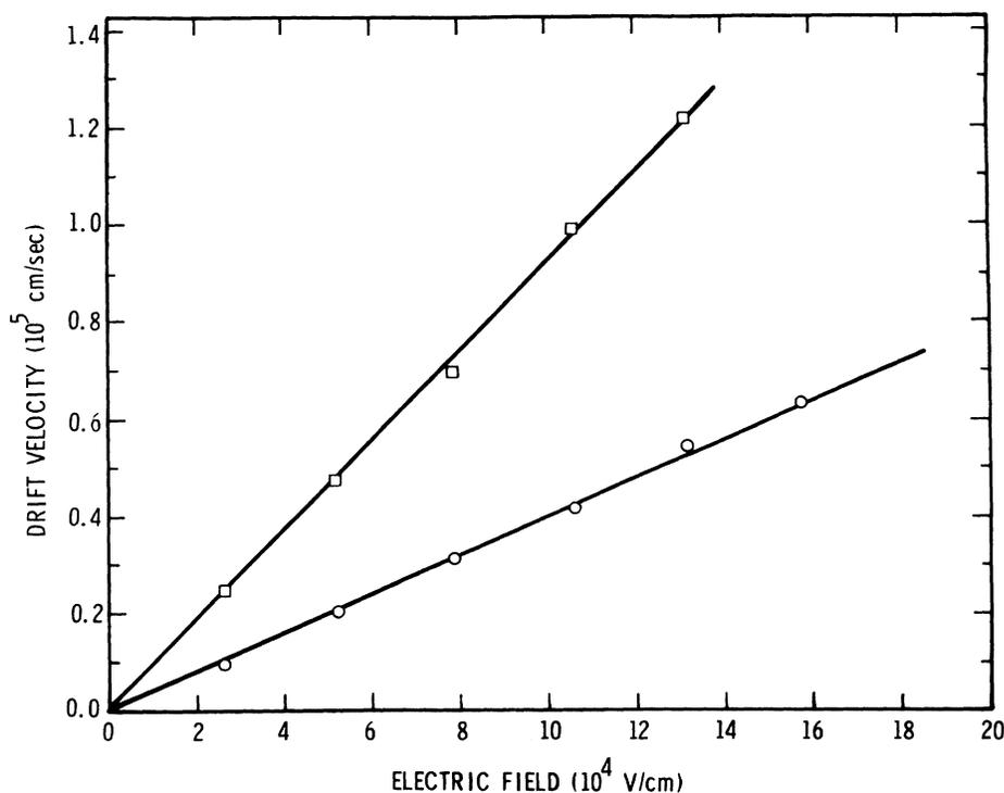
FIG. 2. Reciprocal of the transit time vs applied electric field for a 190- $\mu\text{m}$ -thick crystal. Squares are the data obtained for holes and circles for electrons.
