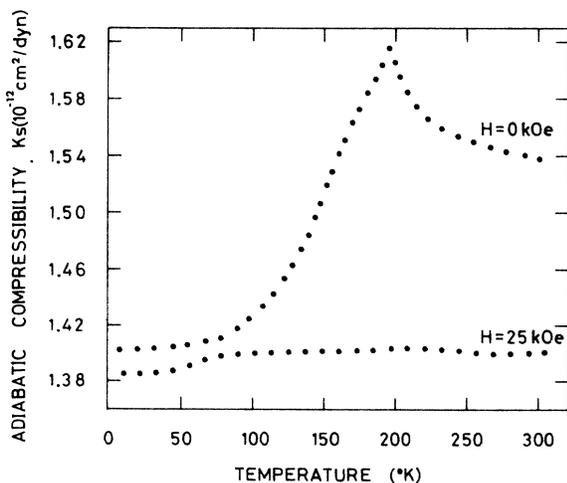
FIG. 2. Temperature dependence of the adiabatic compressibility ( $K_s$ ) of  $\text{SmFe}_2$ , as a function of temperature at zero magnetic field and at 25 kOe.
