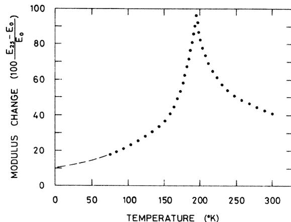
FIG. 4. Relative change in elastic modulus  $(E_{25} - E_0)/E_0$  of  $\text{SmFe}_2$ , as a function of temperature.  $E_0$  and  $E_{25}$  denote the Young moduli at zero magnetic field and at 25 kOe, respectively.
