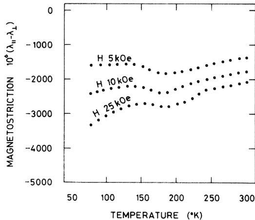
FIG. 5. Temperature and magnetic field dependence of magnetostriction in  $\text{SmFe}_2$ .  $\lambda_{\parallel}$  and  $\lambda_{\perp}$  are the magnetostrains parallel and perpendicular to the applied magnetic field direction, respectively.
