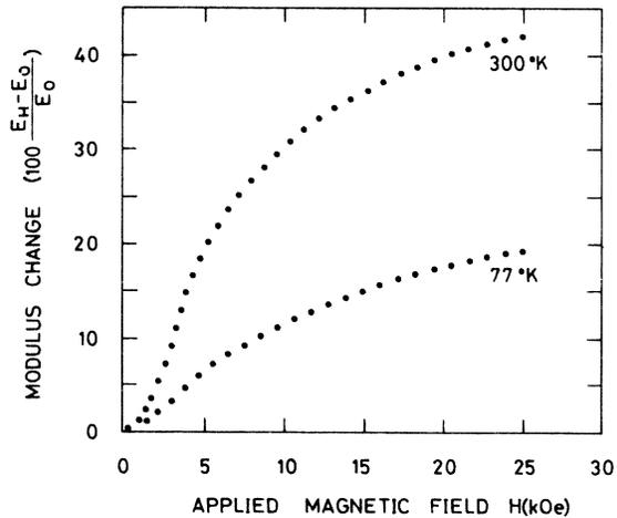
FIG. 3. Relative change in elastic modulus  $(E_H - E_0)/E_0$  of  $\text{SmFe}_2$  at 77 and 300°K, as a function of applied magnetic field.  $E_H$  and  $E_0$  are the magnetized and unmagnetized Young moduli, respectively.
