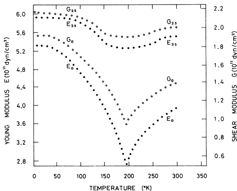
FIG. 1. Temperature dependence of the Young ( $E$ ) and shear ( $G$ ) moduli of  $\text{SmFe}_2$ , as a function of temperature at zero magnetic field and at 25 kOe.
