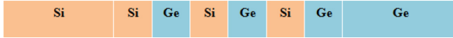
FIG. 1. (Color online) Schematic of the system setup: the left reservoir is pure Si, the right reservoir is pure Ge, the center region is the Si/Ge superlattices.
