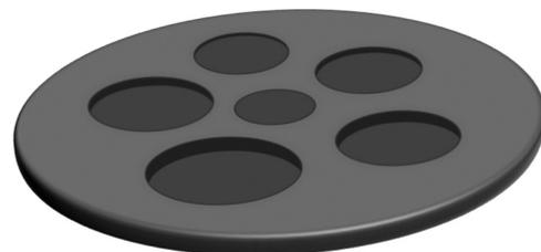
FIG. 3. The Mo baseplate has six pockets of varying depth. Positions of the pockets are optimized to remove side release effects in the data. Each pocket is imaged at two spots near the pocket center, with each spot roughly  $200 \mu\text{m}$  in diameter. The impactor approaches from the flat underside of the target, obscured in this view. The pocket diameters vary from 6 to 10 mm. Baseplate diameter is 32 mm.
