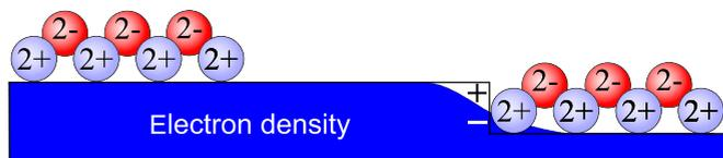
FIG. 4. (Color online) Schematic side view of EuO(111) bilayer islands at a substrate step edge (light blue: Eu; red: O). The indicated charges correspond to the idealized oxidation states in bulk EuO. The electron density of the substrate (indicated in blue) is smoothed at the step edge, leading to a step edge dipole which attracts the polar EuO bilayer at the ascending step edge and repels it at the descending step edge.
