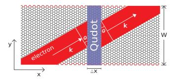
FIG. 1. (Color online) Schematic diagram of an electron elastic scattering with an incident angle  $\theta$ , on a rectangular QD of  $\Delta x$  length.
