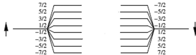
FIG. 2. Splitting of the electronic Ising states into electronuclear states due to the “longitudinal” part of the HF interaction ( H_{\text{HF}}^{\parallel} ). Illustration taken from Schechter and Stamp [22].
