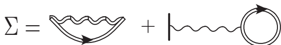
FIG. 2. Contribution to the self-energy from the GW approximation and Hartree diagram. Double wiggly line, single wiggly line, and double line correspond to dressed interaction, bare interaction, and dressed Green's function, respectively.
