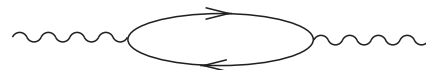
FIG. 2. Feynman diagram representing the vacuum polarization. The wiggly lines represent photons, and the internal lines represent fermionic propagators.
