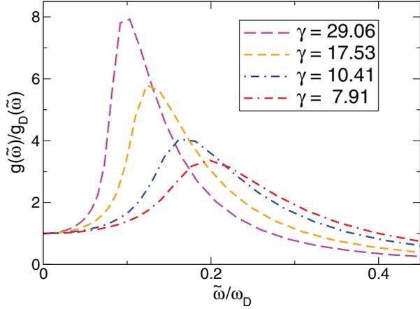
FIG. 3. (Color online) Reduced density of states  $g(\tilde{\omega})/g_D(\tilde{\omega})$  for inverse-power-law disorder with the same disorder parameters as in Figs. 1 and 2. As the disorder increases so does the height of the boson peak; it is also shifted to lower frequencies.
