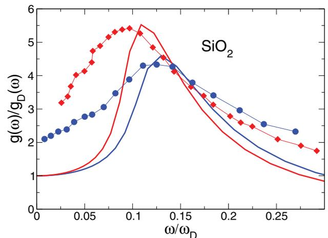
FIG. 6. (Color online) Boson peak data for  $\text{SiO}_2$ <sup>81</sup> compared with the reduced DOS for the inverse-power model with two different lower cutoffs  $\mu$ .
