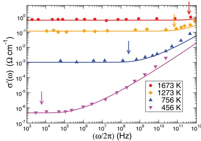
FIG. 1. (Color online) Comparison of ionic ac conductivity data of sodium trisilicate glass<sup>73</sup> with the CPA prediction for activated hopping with a constant-barrier distribution. We use units in which  $D_0 = k_\xi = 1$ . The arrows indicate the boson-peak positions  $\omega_{\text{BP}} \equiv \tilde{\omega}_{\text{BP}}^2$  of Fig. 3.
