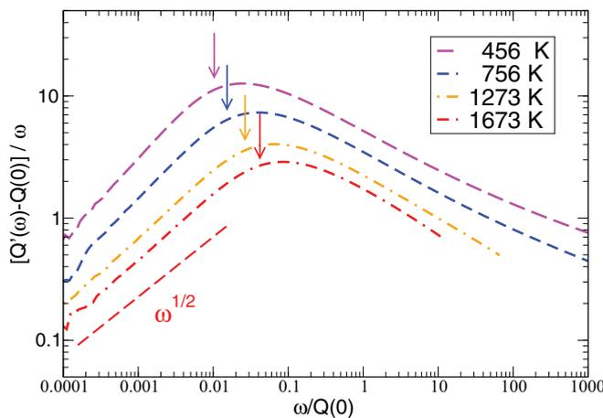
FIG. 2. (Color online) Loss function  $[Q'(\omega) - Q(0)]/\omega \propto [\sigma(\omega) - \sigma(0)]/\omega$  calculated from the CPA curves in Fig. 1. Below the dc-ac crossover the Rayleigh-type nonanalyticity is visible.
