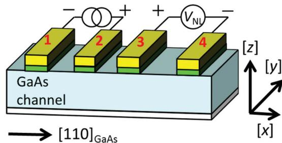
FIG. 1. (Color online) Schematic device structure of a four-terminal lateral spin-transport device and circuit configuration for nonlocal measurements.
