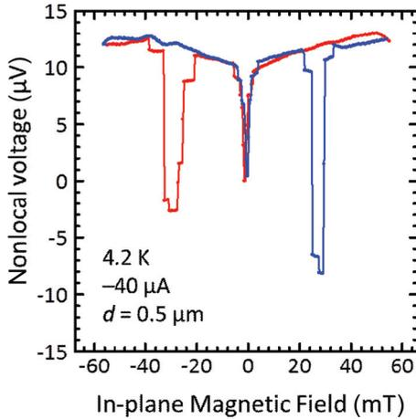
FIG. 2. (Color online) Plot of nonlocal voltage as a function of in-plane magnetic field ( $B_x$ ) for a lateral spin-transport device with  $\text{Co}_2\text{MnSi}/\text{CoFe}/n\text{-GaAs}$  junctions. A background signal consisting of a constant term and linear and quadratic terms of  $B_x$  has been subtracted.
