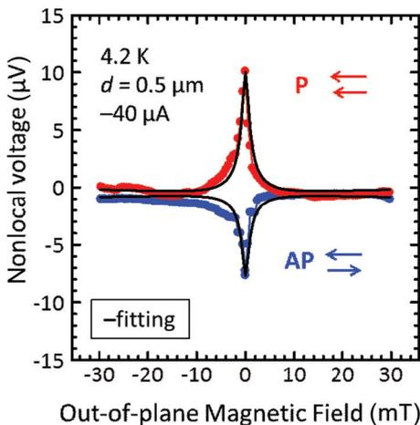
FIG. 3. (Color online) Plot of nonlocal voltage as a function of out-of-plane magnetic field ( $B_z$ ) for a  $\text{Co}_2\text{MnSi}/\text{CoFe}/n\text{-GaAs}$  sample for both P (upper curve) and AP (lower curve) configurations. The solid lines are the result of the fitting using Eq. (1).
