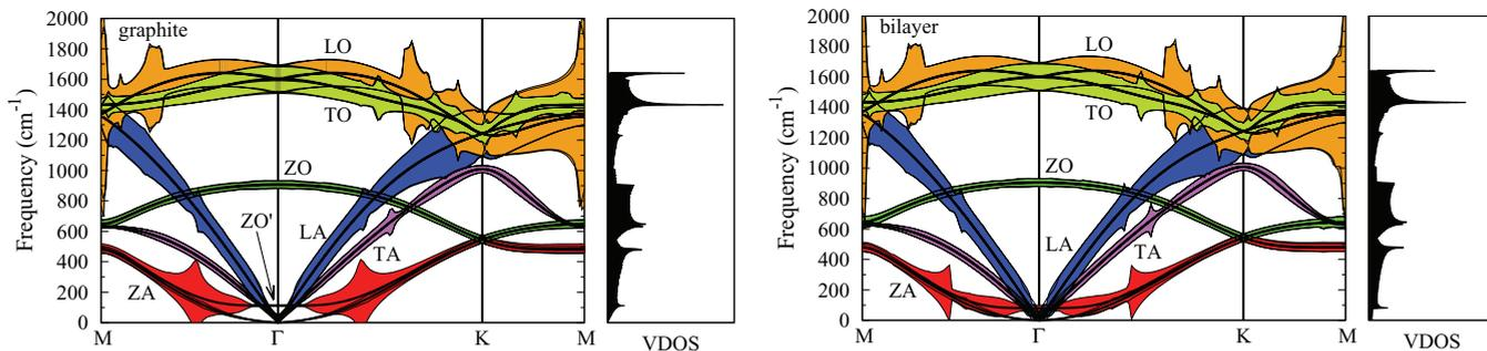
FIG. 8. (Color online) Graphite and graphene bilayer: calculated phonon dispersion widened by the anharmonic broadening (FWHM  $\times 100$ ) at 300 K.
