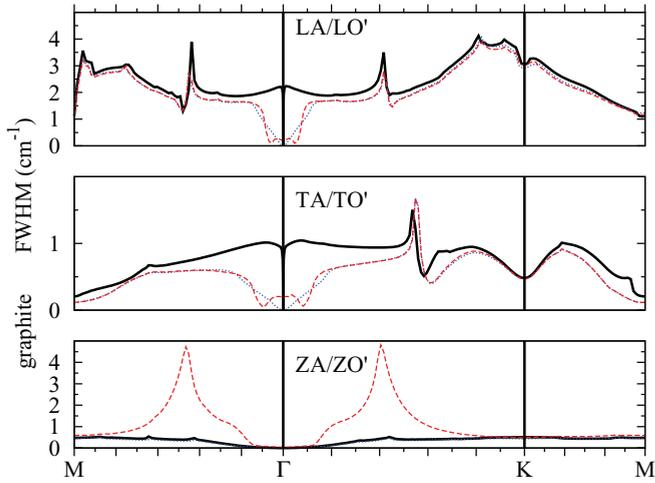
FIG. 9. (Color online) Anharmonic phonon broadening (FWHM) at 300 K. Graphene acoustic branches (solid line) are compared with the corresponding graphite acoustical (dotted) and quasiacoustical (dashed) ones.
