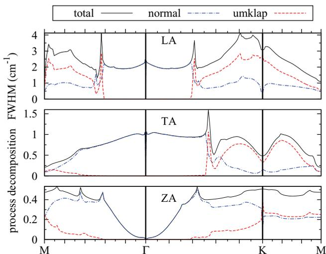
FIG. 4. (Color online) Graphene anharmonic phonon broadening for the three acoustic branches at 300 K (same data as in Fig. 3): the broadening is decomposed in two components, which are due, respectively, to normal and umklapp processes.
