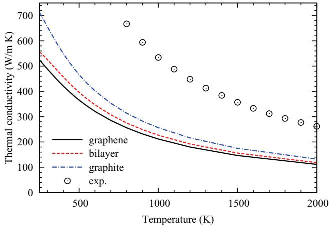
FIG. 13. (Color online) In-plane thermal conductivity calculated within the SMA for graphene single and bilayer and bulk graphite. Measurements (exp.) are done on graphite and are from Ref. 29.
