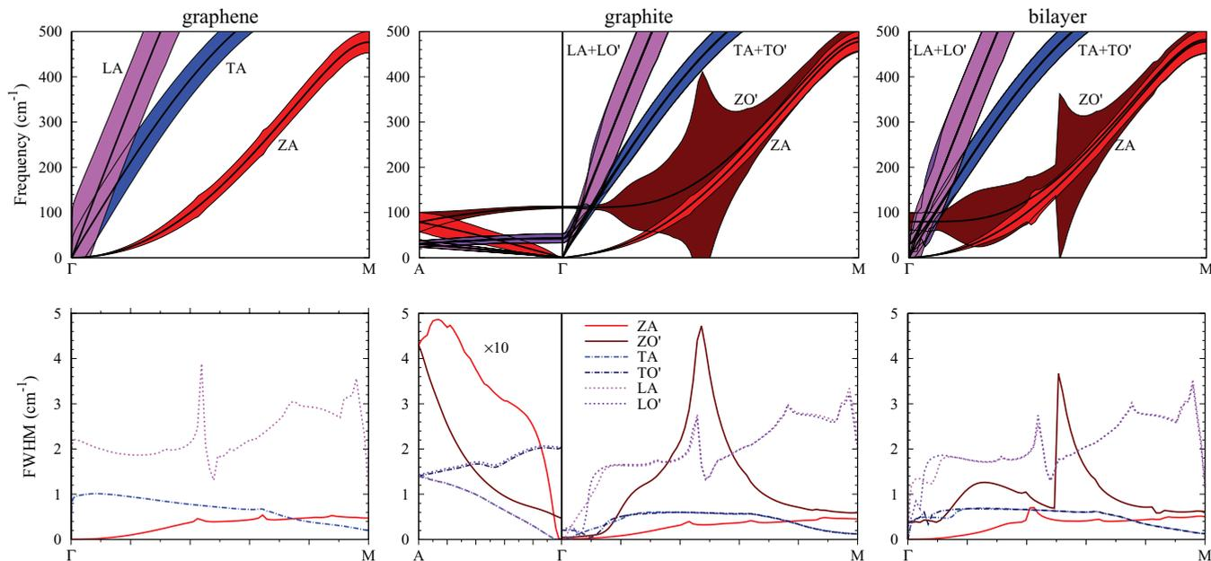
FIG. 11. (Color online) Phonon dispersion and anharmonic broadening of the acoustic and quasiacoustic branches of graphene, graphite, and graphene bilayer. The upper panels show the lower part of the phonon dispersion as in Figs. 2 and 8. The lower panels show the FWHM at 300 K. The values in the A- $\Gamma$  section for graphite are magnified by a factor 10.
