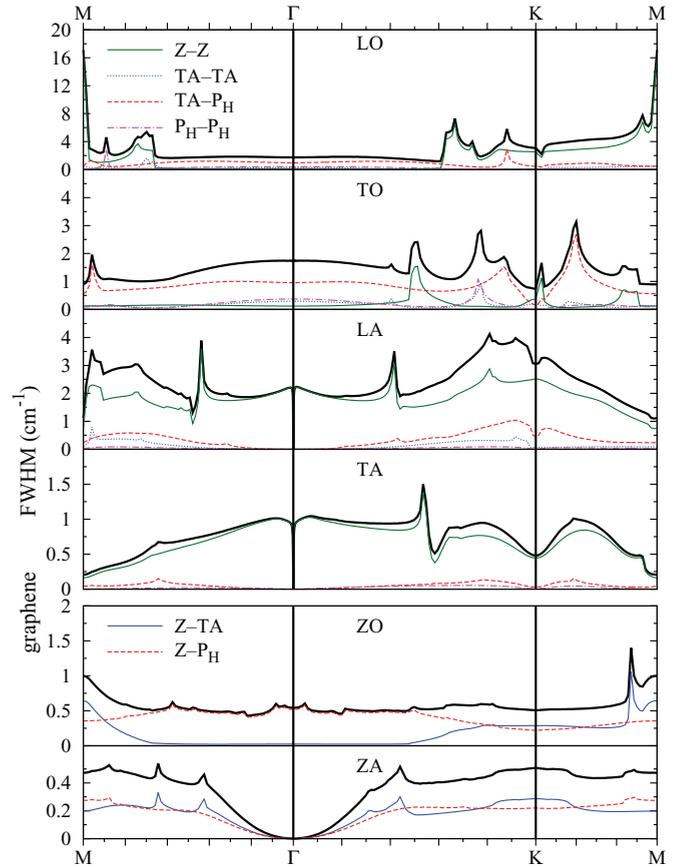
FIG. 3. (Color online) Graphene anharmonic phonon broadening (FWHM) at 300 K, for each phonon branch (labeled as in Fig. 2), along high-symmetry lines. The total broadening (solid thick line) is decomposed depending on the character of the final states, which are labeled as Z, TA, and  $P_H$  (see the text), e.g., TA- $P_H$  corresponds to a decay involving one TA and one  $P_H$  phonons.
