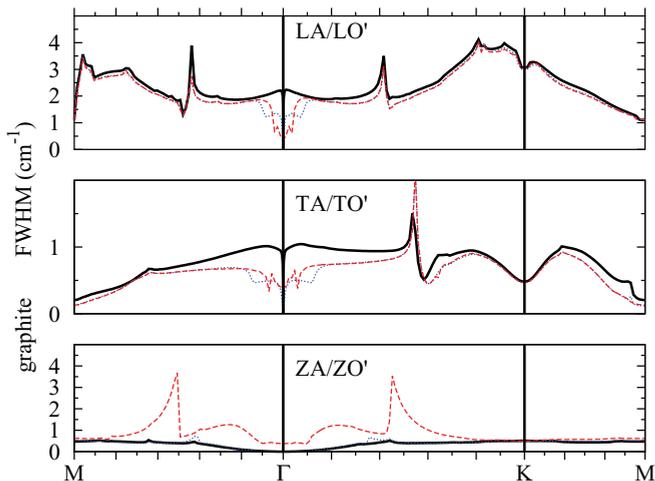
FIG. 10. (Color online) Anharmonic phonon broadening (FWHM) at 300 K. Graphene monolayer acoustic branches (solid line) are compared with the corresponding bilayer acoustical (dotted) and quasiacoustical (dashed) ones.
