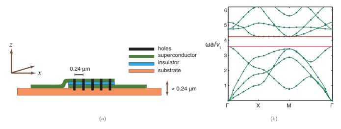
FIG. 3. (Color online) (a) The proposed design of the qubit. Note that the holes are drilled in a square lattice pattern at regular intervals of 0.24  $\mu$ m and the qubit must be fabricated on a substrate no greater than the same length, (b) The band structure for  $k_z = 0$ .  $\Gamma$ , X, and M represent the points ( $k_x a, k_y a$ ) = (0,0), (0, $\pi$ ), and ( $\pi$ , $\pi$ ), respectively. The band gap extends from  $\omega a/v_t = 3.57$  to  $\omega a/v_t = 4.23$ .
