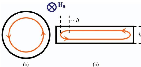
FIG. 2. (Color online) Foucault current density scale in (a) sphere and (b) disk.
