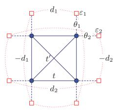
FIG. 1. (Color online) Cluster and bath parametrization used in this work. Hopping terms are shown by solid lines, bath hybridization by dashed lines, and bath pairing terms by dotted lines.
