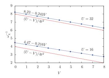
FIG. 2. (Color online) Blue dots: Inverse frequency of the dominant peak in the antiferromagnetic susceptibility of the extended Hubbard model at half filling, as a function of the nearest-neighbor interaction V, for U=16 and U=32 (t=1). These inverse frequencies are expected to be  $J^{-1}=(U-V)/4t^2$  in the large-U limit
