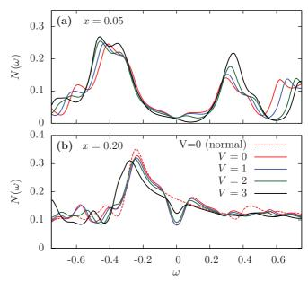
FIG. 7. (Color online) Local density of states for four values V = 1,2,3,4 and U = 8 for (a) underdoped x = 0.05, and (b) overdoped x = 0.2 regimes. The dotted line in (b) is for the normal state V = 0, all other lines in (a) and (b) are for the superconducting state.
