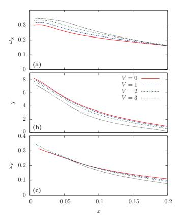
FIG. 6. (Color online) (a) Position of the lowest peak in the AF susceptibility  $\chi''(\omega)$  and the strength  $\chi$  of that peak in (b), for U = 8. (c) shows the corresponding superconducting (SC) characteristic frequency  $\omega_F$ .
