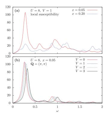
FIG. 4. (Color online) (a) Imaginary part of the local spin susceptibility  $\chi''(\omega)$  for U=8, V=1 for an underdoped (x=0.05) and an overdoped (x=0.20) case. (b) In the underdoped regime (x=0.05) apart from a shift of the low-frequency peak to higher frequencies, it is mostly the amplitude, not the structure of the imaginary part of the plaquette antiferromagnetic spin susceptibility  $\chi''(\mathbf{Q},\omega)$ , that is slightly affected by V.
