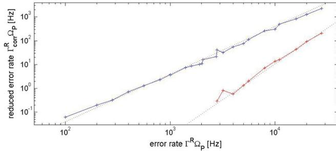
FIG. 3. (Color online) Corrected error rates with respect to time for three (upper curve) and five (lower curve) pump circuits as a function of the uncorrected error rates. Dashed lines are a fit to Eq. (1). Other parameters as in Fig. 2.
