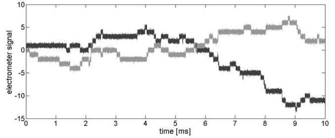
FIG. 2. Signal traces of first (black) and second (gray) electrometer. Pump error rates are 1000/s, per pump and sign, electrometer noise  $10^{-5}e/\sqrt{\text{Hz}}$ , and coupling capacitance ratio  $C_C/C_{\text{node}} = 0.04$ .
