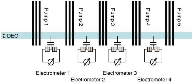
FIG. 1. (Color online) Schematic of a circuit for an error-correction scheme in a typical electron counting experiment composed of metallic single-electron transistors and electron pumps utilizing dynamic quantum dots in a two-dimensional electron gas.
