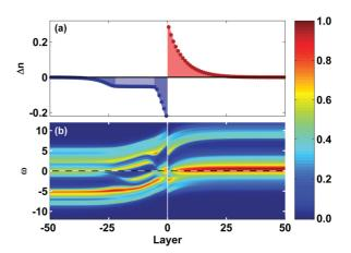
FIG. 4. (Color online) (a) Charge redistribution as a function of the plane number (the z axis) of the structure (U=8t,  $\Delta e_f=-7t$ ,  $e_C=0.1t$ ). (b) Color coded DOS in arbitrary units as a function of  $\omega$  and the plane number. The Fermi level in the DOS is at  $\omega=0$  (dashed line). We observe an insulating region several planes wide, where n=1.
