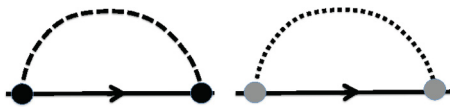
FIG. 1. Self-energy diagrams. The solid line is the bare quasiparticle propagator, the dashed (dotted) lines represent the charge (spin) collective mode propagators, Eq. (1), with \lambda = C(S) . The black and gray dots represent the couplings of quasiparticles with charge and spin collective modes g_C and g_S , respectively.
