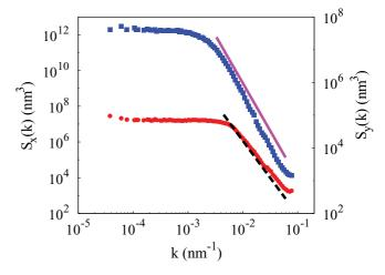
FIG. 6. (Color online) PSD of one-dimensional cuts  $S_x(k)$  (red circles, left axis) and  $S_y(k)$  (blue squares, right axis) of the samples illustrated in Fig. 4, after an average over seven windows. The black dashed line and the solid magenta line correspond to Eqs. (9) and (10), respectively, with exponents values given by Eq. (21).
