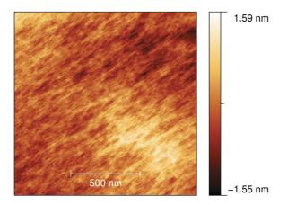
FIG. 1. (Color online) STM top views of the surface morphology for the contamination-free sample. Image size is  $1.3 \times 1.3 \ \mu m^2$ .
