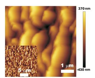
FIG. 4. (Color online) AFM top view of the morphology of Si(100) irradiated for 8 h with 40 keV  $Ar^+$  ions and concurrent Fe codeposition. Image size is  $6 \times 6 \ \mu m^2$ .
