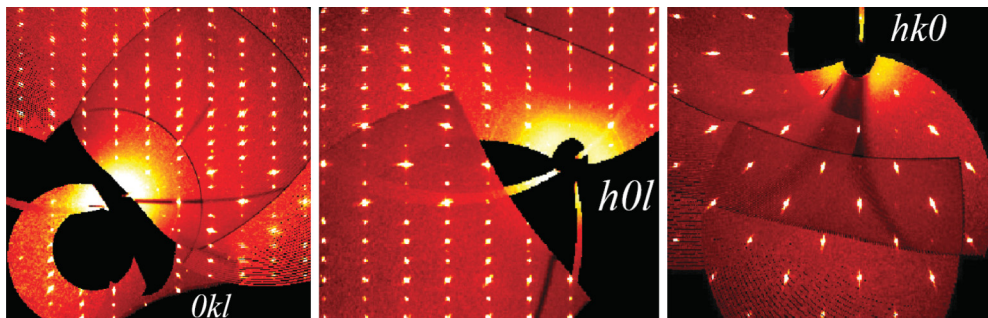
FIG. 4. (Color online) The reconstructed Ok_l , hO_l , and hk_0 reciprocal space sections of the single-crystal SmFe_{0.92}Co_{0.08}AsO .
