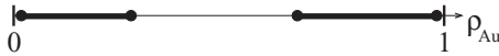
FIG. 3. Stability diagram of a Si(111) surface, with an uphill current ( \delta > 0 ), when doped with a variable quantity of Au. The clean surface ( \rho_{\text{Au}} = 0 ) and the fully covered Si surface ( \rho_{\text{Au}} = 1 ) are stable. A tiny Au deposition on the clean surface or a tiny removal of it from the fully covered surface induces a stability reversal and the surface becomes unstable (thick horizontal lines). In the intermediate region, the surface is expected to recover stability (thin horizontal line), because the Au profile is more flat. If the sign of the current is reversed, stability regions are also reversed (thick line \leftrightarrow thin line).
