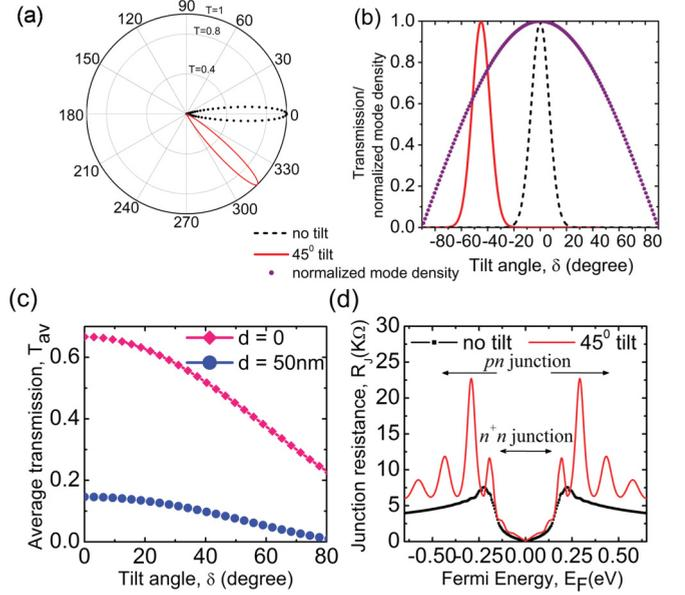
FIG. 2. (Color online) (a) Angular transmission for various tilt angles. (b) With tilt, the transmission lobe moves into a low angular mode density ( $\sim \cos \theta$ ) area, giving (c) a gradual decrease in transmission [Eq. (3)] for a symmetric  $p$ - $n$  junction. (d) Junction resistance at 0 K predicted from Eq. (4). We see resonances which become more pronounced as we go into smaller systems.
