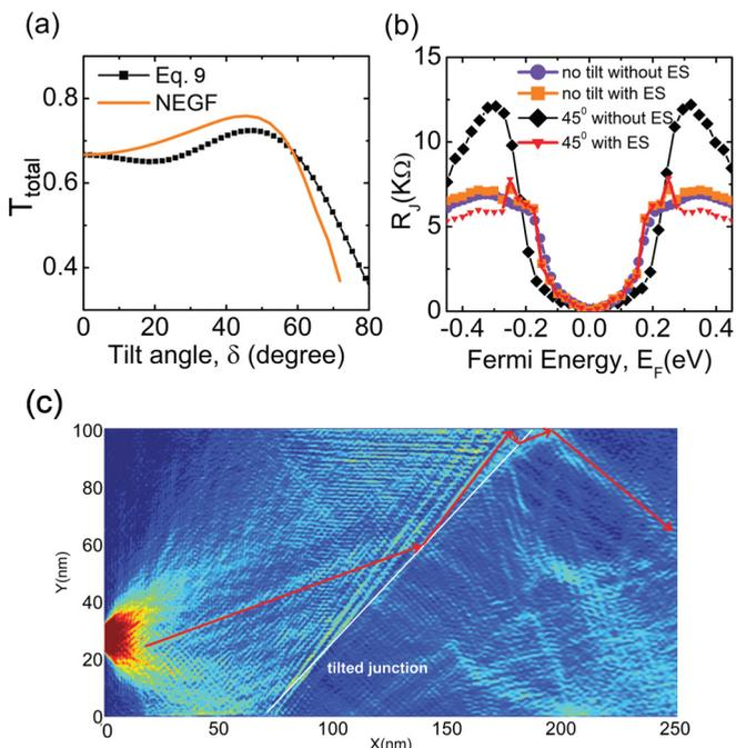
FIG. 4. (Color online) (a) Increase in conductance in a tilted GPNJ due to edge scattering (ES) in contrast with Fig. 2(c). (b) Corresponding decrease in junction resistance due to tilt. (c) Mechanism of edge enhanced conductance for a tilted junction from an atomistic NEGF calculation. We put a small source (bright red spot)—some reflected electrons are incident at the junction again after edge reflection.
