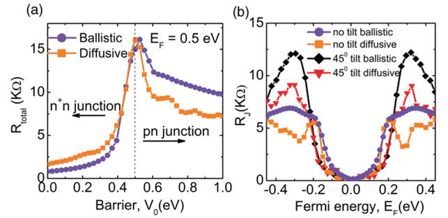
FIG. 3. (Color online) Impact of charged impurity scattering. (a) Conductance asymmetry is diluted due to impurity potentials, and the ballistic resistance is normalized for comparison. (b) Reduced asymmetry results in a lower junction resistance for both tilted and nontilted devices, thus retaining their difference.
