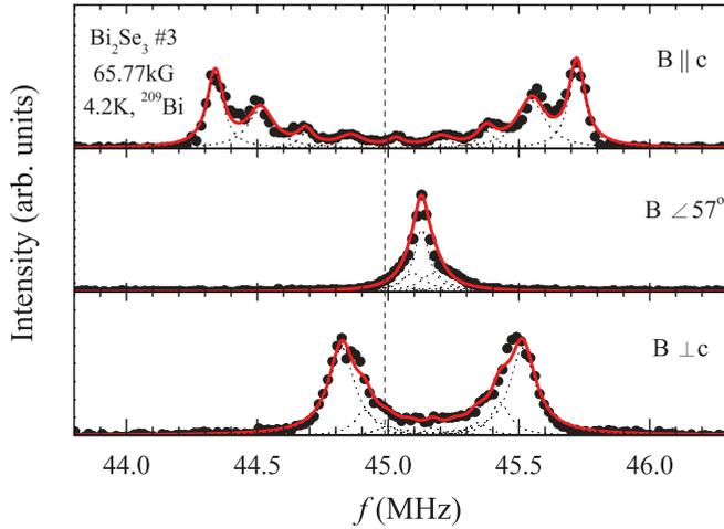
FIG. 3. (Color online) The curve fittings for the  $^{209}\text{Bi}$  NMR frequency-swept spectra of  $\text{Bi}_2\text{Se}_3$ , sample No. 3, for the magnetic field directions  $B \parallel c$ ,  $B \angle 57^\circ$ , and  $B \perp c$ . (Circles: spectrum points; red curve: fitting curve; dotted curve: individual quadrupolar peaks.)
