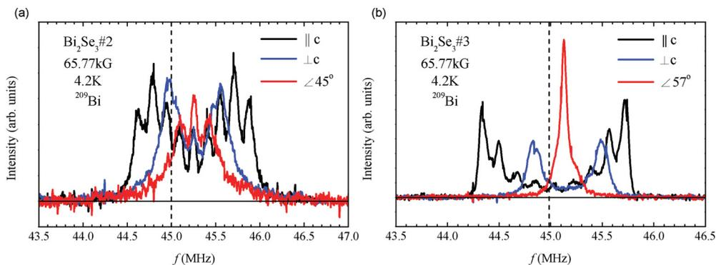
FIG. 2. (Color online)  $^{209}\text{Bi}$  NMR frequency-swept spectra of  $\text{Bi}_2\text{Se}_3$  for (a) sample No. 2 and (b) sample No. 3, with magnetic fields applied at different angles with respect to the  $c$  axis. The dashed line denotes the unshifted Larmor frequency position.
