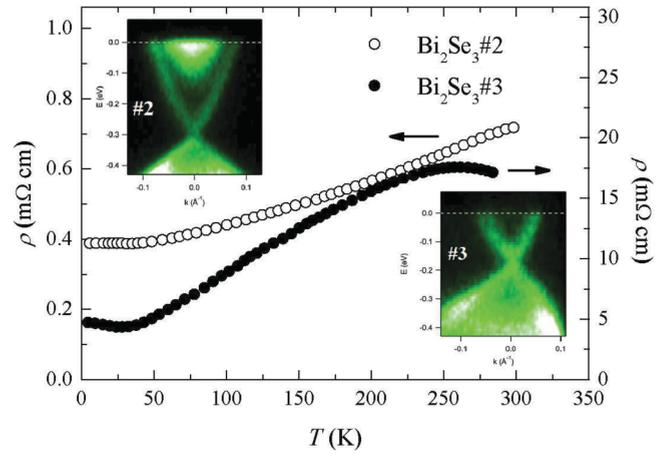
FIG. 5. (Color online) Temperature-dependent resistivity for  $\text{Bi}_2\text{Se}_3$  samples No. 2 (open circles) and No. 3 (solid circles). The corresponding ARPES spectra (insets) show a significant shift in the chemical potential between these two samples, indicating higher carrier concentration in sample No. 2. The spectra were recorded along the  $\Gamma\text{K}$  line in the surface Brillouin zone.
