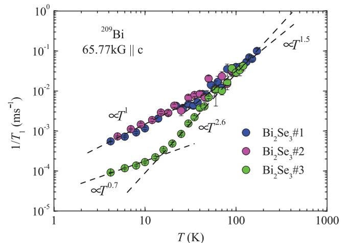
FIG. 6. (Color online) Temperature dependence of nuclear spin-lattice relaxation rate ( $1/T_1$ ) for  $\text{Bi}_2\text{Se}_3$  crystals.
