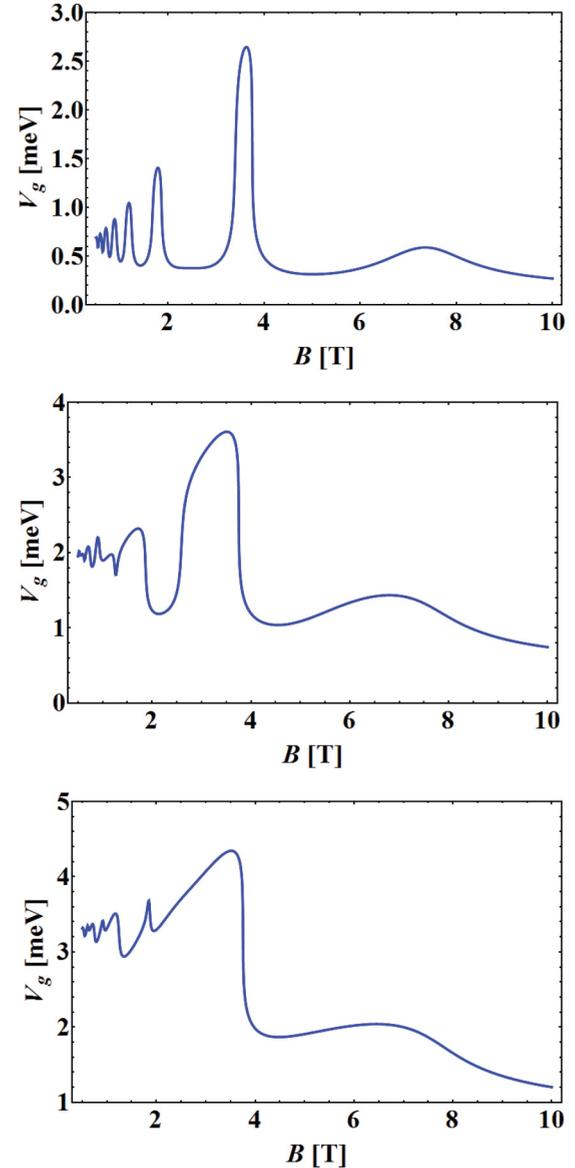
FIG. 2. (Color online) Screened gating potentials as a function of magnetic field: We show results for bare gateings of 10 meV, 30 meV, and 50 meV. Low/high screening does not directly correspond to transition/plateau regions of  $R_{xy}$  as broadened LLs for different spin significantly overlap for the Zeeman energy found.
