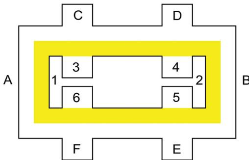
FIG. 1. (Color online) Geometry of the anti-Hall bar within a Hall bar: The figure shows the labeling of contacts used and the shaded, yellow area denotes the partial gating applied by a top gate in the experiment.
