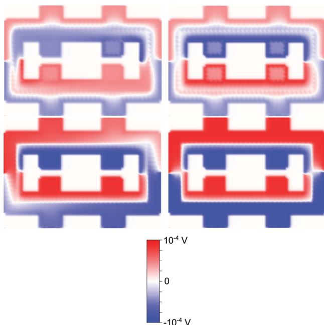
FIG. 5. (Color online) Distribution of the electrochemical potential: We show results for a bare gating potential of 30 meV and magnetic field values (from top left to bottom right) of 3.66 T, 4.20 T, 4.86 T, and 5.50 T.
