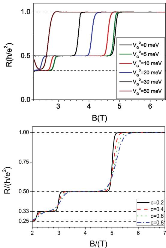
FIG. 3. (Color online) Variation of the transversal resistances as a function of magnetic field: The upper plot shows  $R_{xy}$  for various gating potentials applied to the inner gated bar. The lower curves show transversal resistance curves for various curvatures  $c$  and no gating.
