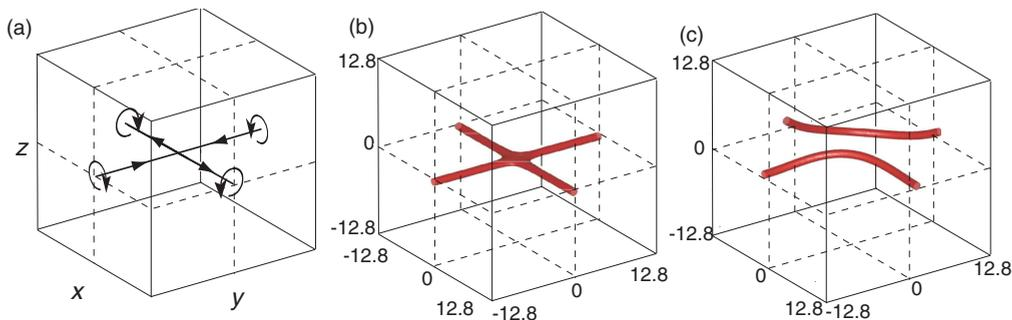
FIG. 3. (Color online) The  $\Psi_4$  reconnection fixed point is shown schematically in (a). It consists of four half-infinite coplanar vortices meeting at right angles. Isosurfaces of the fixed point at  $|\Psi_4| = 0.3$  are shown in (b), as obtained via the diffusive GP equation. The fixed point is, dynamically, an exponentially unstable saddle that, after a minimal white-noise perturbation in a time-dependent GP solver, develops with time in a box of size  $L = 24.6$  as shown in part (c).
