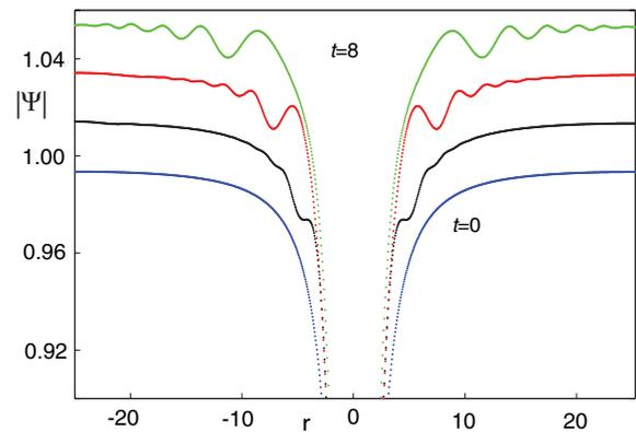
FIG. 2. (Color online) Time evolution of the Fetter approximant for a single straight stationary vortex according to the GPE integrated in a periodic domain:  $f_F = |\Psi|$  is plotted at times  $t = 0, 2, 4, 8$  along a midplane section. To reveal the time evolution, successive profiles have been shifted. Evidently, the density profile  $f_F$  is not a minimal-energy condition and immediately launches erroneous acoustic waves.
