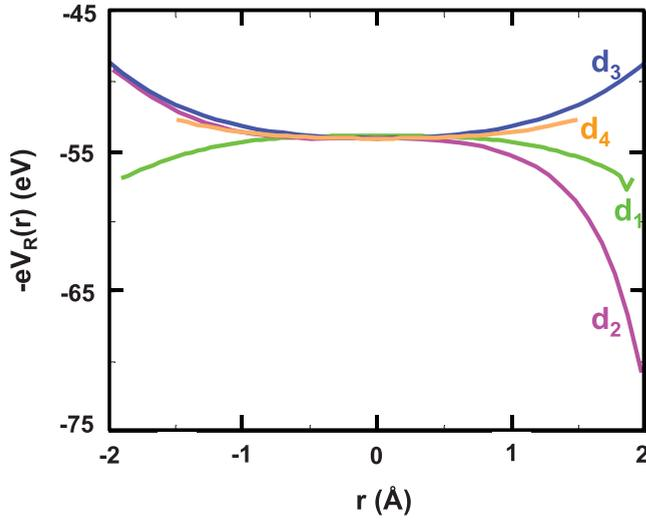
FIG. 5. (Color online) Potential energy  $(-e)V_R(\mathbf{r})$  for emerald. Energy is depicted along  $d_1$ ,  $d_2$ ,  $d_3$ , and  $d_4$  directions corresponding, respectively, to a O–Cr–O path joining two opposite oxygens, a  $C_2$  axis joining  $\text{Cr}^{3+}$  with a close  $\text{Be}^{2+}$ , the  $C_3$  axis, and a path bisecting a O–Cr–O angle involving two adjacent oxygens which does not intersect a close  $\text{Be}^{2+}$  ion (Fig. 4).
