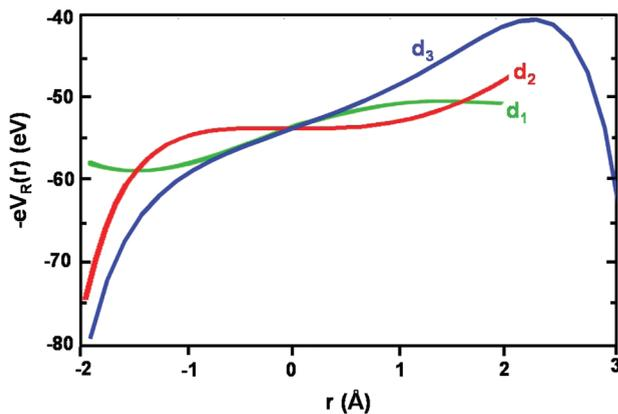
FIG. 2. (Color online) Potential energy on an electron,  $(-e)V_R(\mathbf{r})$ , due to the internal electric potential,  $V_R(\mathbf{r})$ , produced by the rest of the lattice ions of ruby on the  $\text{CrO}_6^{9-}$  complex. Energy is depicted along the  $\text{O}_s\text{-Cr-O}_l$  path (direction  $d_1$ ), the diagonal joining the central  $\text{Cr}^{3+}$  impurity, and one  $\text{Al}_1^{3+}$  cation (direction  $d_2$ ) and the  $C_3$  axis (direction  $d_3$ ).
