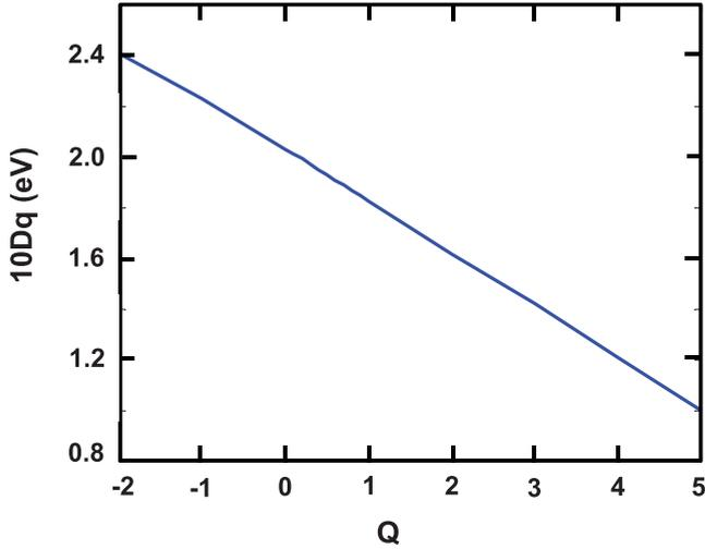
FIG. 7. (Color online) Calculated values of 10Dq as a function of the external charge  $Q$  for the model system. The external charges are placed at a distance  $R_q = 4 \text{ \AA}$  from the chromium ion.
