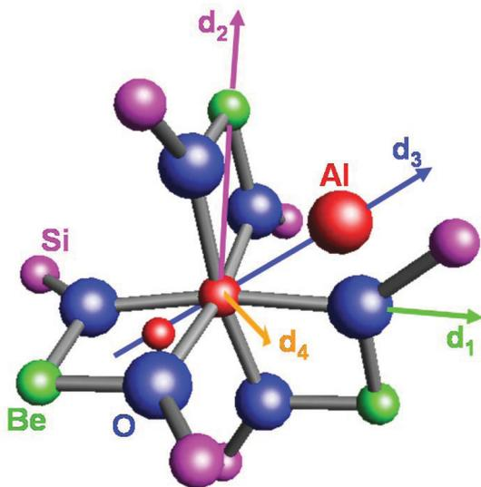
FIG. 4. (Color online) Local structure of beryl ( $\text{Be}_3\text{Si}_6\text{Al}_2\text{O}_{18}$ ) around an  $\text{Al}^{3+}$  ion with a  $D_3$  symmetry. All nearest  $\text{O}^{2-}$  anions lie at the same distance  $R = 1.903$  Å.
