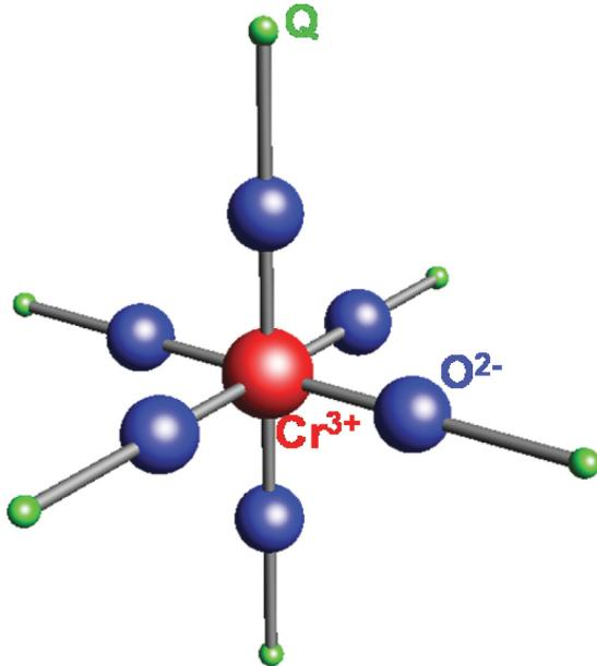
FIG. 6. (Color online) Model system formed by an octahedral  $\text{CrO}_6^{9-}$  complex surrounded by six identical point charges  $Q$  at the same distance  $R_q$  from the chromium ion and placed along the three  $C_4$  axes of the octahedron.
