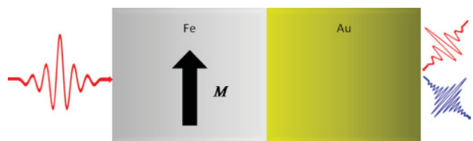
FIG. 3. (Color online) Schematic setup of the optical pump-probe experiment on a Fe/Au heterostructure.
