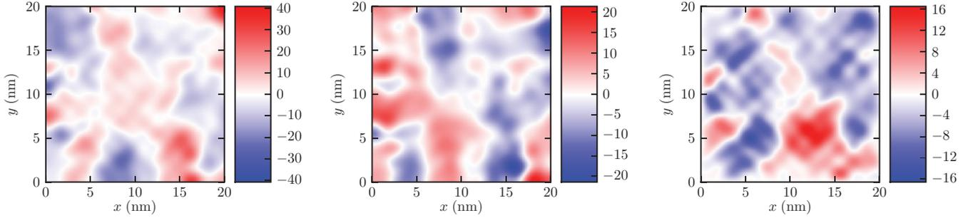
FIG. 2. (Color online) Left: Color/grayscale plot of the scalar potential  $V_1(\mathbf{r})$  (in units of meV) calculated using Eq. (4) with  $g_1 = 3$  eV. Center: The  $\hat{x}$ -component  $A_x(\mathbf{r})$  of the vector potential (in units of meV) calculated using Eq. (4). Right: Same as in the central panel but for the  $\hat{y}$ -component  $A_y(\mathbf{r})$  of the vector potential.
