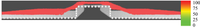
FIG. 5. (Color online) The optimum configuration of armchair graphene over an elongated cubic barrier with |x| < 1.5 nm where the zigzag edges were supported in the x - y plane. The colors indicate the size of strain.
