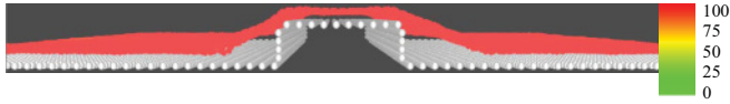
FIG. 9. (Color online) The optimum configuration of armchair graphene over an elongated barrier of size |x| < 1.5 nm where zigzag edges were supported in the x - y plane (see also Fig. 8 which shows graphene with free boundaries over the same substrate). Here \epsilon = 10 meV and \sigma = 3.4 Å for 12-6 LJ potential.
