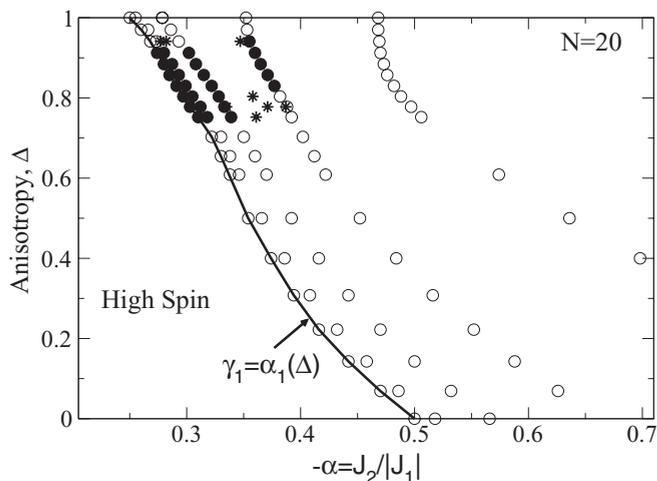
FIG. 2. Parameter points  $(\alpha, \Delta)$  for a doubly degenerate GS of  $H(\alpha, \Delta)$  [Eq. (1)] with  $N = 20$  spins. Open circles indicate inversion degeneracy  $C_i = \pm 1$ , closed circles indicate spin-parity degeneracy  $P = \pm 1$ , and stars indicate vector chiral degeneracy  $C_i, P = \pm 1$ . The line  $\alpha_1(\Delta)$  marks degeneracy between high and low spin.
