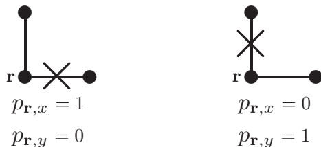
FIG. 1. The occupation number p_{r,\alpha} ( \alpha = x, y ) takes value 1 if bond (\mathbf{r}, \mathbf{u}_\alpha) is removed and 0 otherwise.
