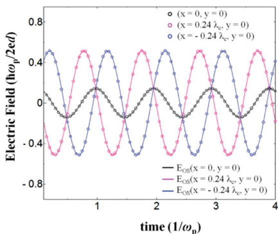
FIG. 5. (Color online) The time evolution of the oscillation part of electric fields at  $V = 6.44V_p$ . The black, red, and blue open circles indicate the calculated values in our simulation at  $(x, y) = (0, 0)$ ,  $(x, y) = (0.24\lambda_c, 0)$ , and  $(x, y) = (-0.24\lambda_c, 0)$ , respectively. The lines indicate  $E_{OS}$  at each position when  $m = 1, n = 0$ ,  $E_{bg} = 0.142$ ,  $E_{cv} = 0.492$ , and  $\varphi_0 = 0.5\pi$ .
