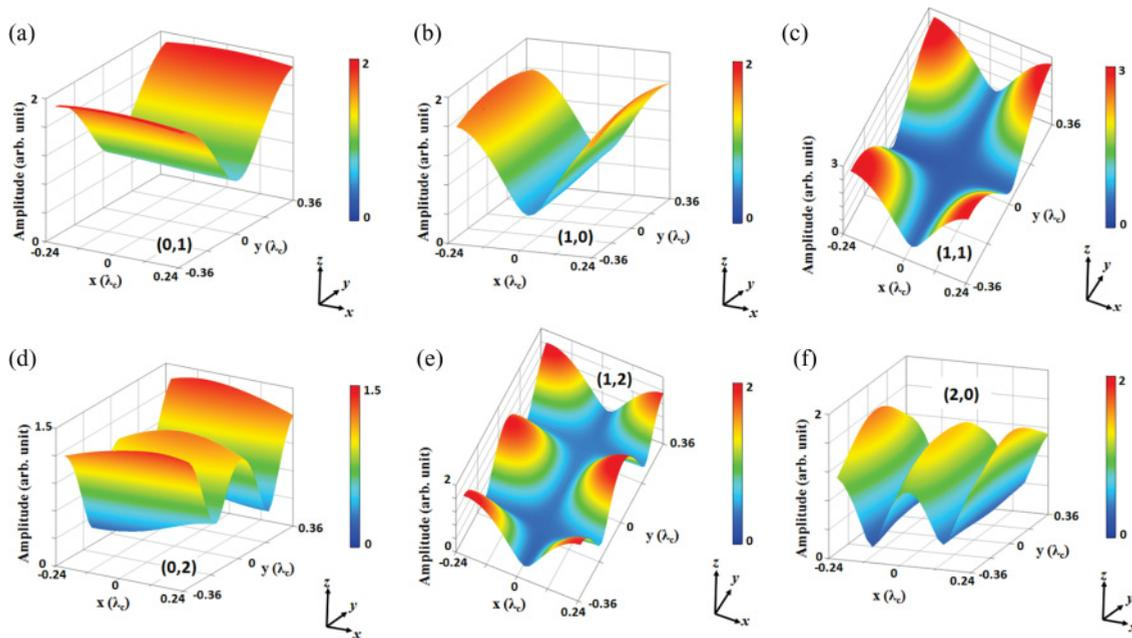
FIG. 4. (Color online) The Fourier components of electric fields  $E_z$  at (a)  $V = 4.47V_p$ , (b)  $V = 6.44V_p$ , (c)  $V = 8.07V_p$ , (d)  $V = 8.77V_p$ , (e)  $V = 11.3V_p$ , and (f)  $V = 12.7V_p$ .
