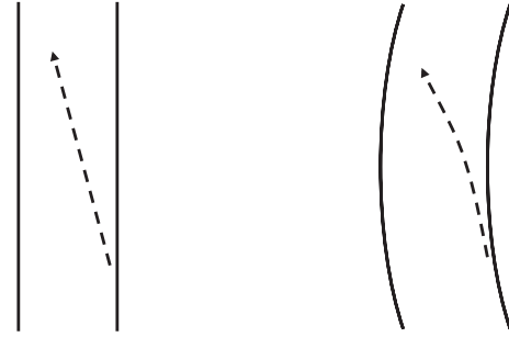
FIG. 4. Schematic diagram showing the effect of bending a plate on phonon propagation. The solid line represents the walls of the plate and the dashed line shows a possible trajectory of a phonon.
