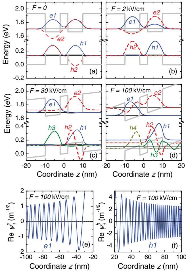
FIG. 2. (Color online) [(a)–(d)] Wave functions and energy levels of electron and hole ground and excited states for different values of the electric field  $F$ . Gray lines show CQW heterostructure potentials, using  $E_g = 1.519$  eV for the band gap. [(e) and (f)] Oscillating tails in the electron and hole wave functions.
