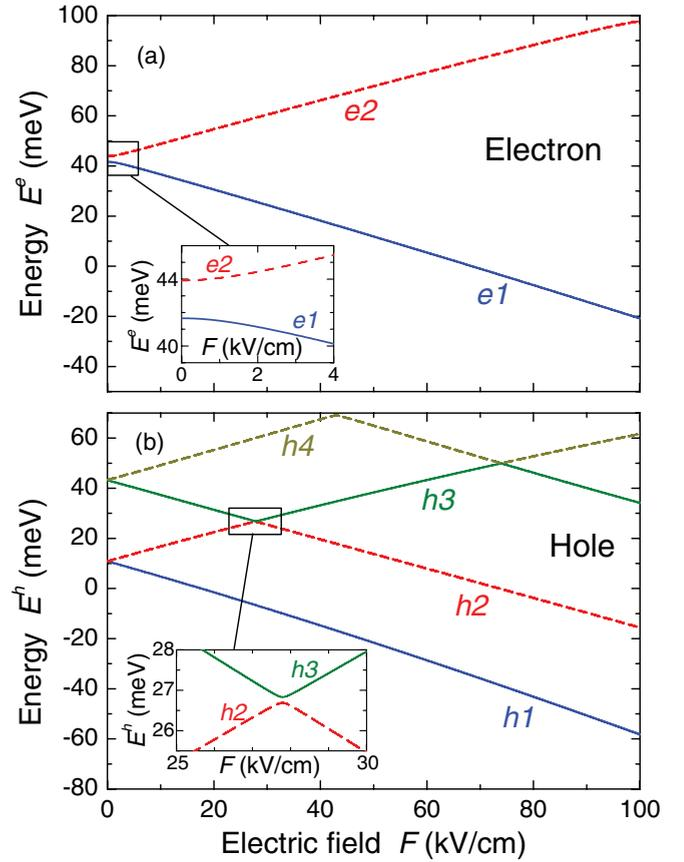
FIG. 1. (Color online) Energies of two electron states (a) and four hole states (b) in 8–4–8-nm GaAs/Al<sub>0.33</sub>Ga<sub>0.67</sub>As CQW as functions of an applied electric field. Insets show spectral regions with anticrossing.
