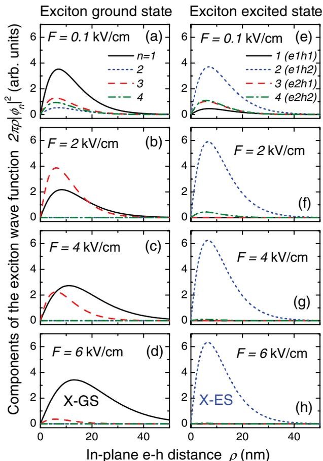
FIG. 6. (Color online) Radial components  $2\pi\rho|\phi_n(\rho)|^2$  of the exciton wave function calculated for the ground state X-GS [(a)–(d)] and excited state X-ES [(e)–(h)] for different values of the electric field.
