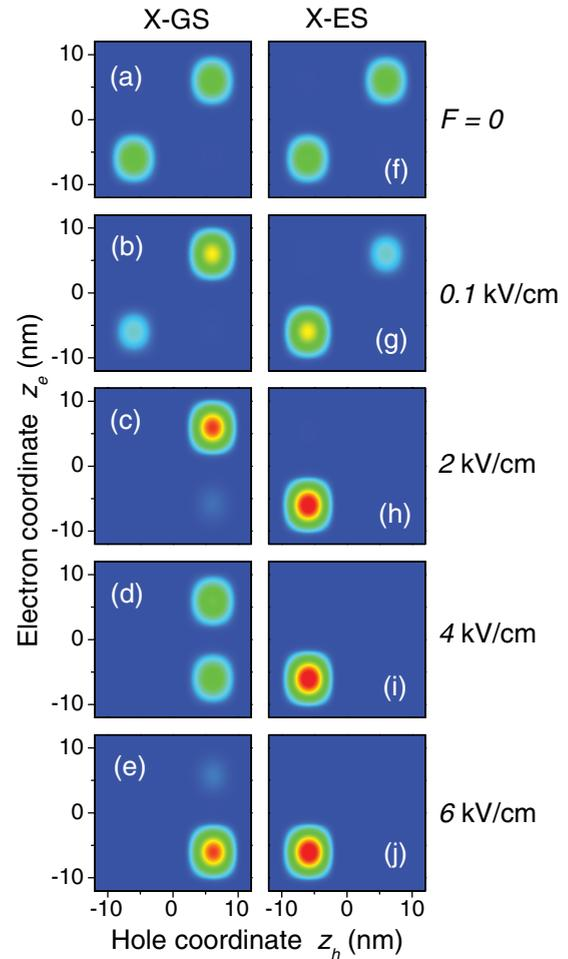
FIG. 5. (Color online) Probability distributions  $\int_0^\infty |\Phi(z_e, z_h, \rho)|^2 2\pi\rho d\rho$  calculated for the exciton ground state X-GS [(a)–(e)] and excited state X-ES [(f)–(j)] for different values of the electric field.
