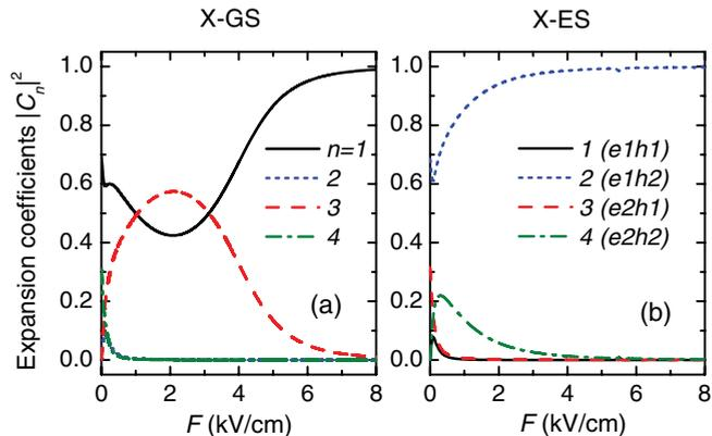
FIG. 7. (Color online) Coefficients  $C_n$  of the expansion of the exciton wave function into e-h pair states calculated for the ground state X-GS (a) and excited state X-ES (b) as functions of the electric field  $F$ .
