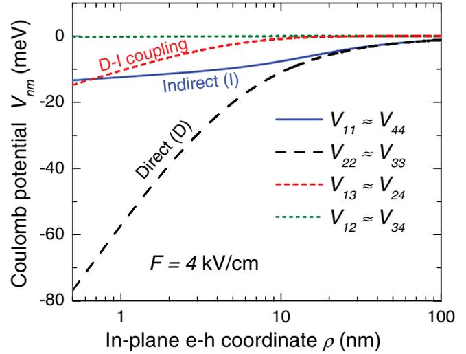
FIG. 3. (Color online) Matrix elements  $V_{nm}$  of the Coulomb potential calculated between different e-h pair states at  $F = 4$  kV/cm.
