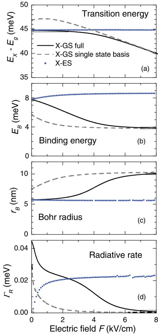
FIG. 8. (Color online) (a) Optical transition energy  $E_X$ , (b) binding energy  $E_b$ , (c) in-plane Bohr radius  $r_B = \sqrt{\langle \rho^2 \rangle}$ , and (d) radiative rate  $\Gamma_R$  of the exciton ground state X-GS (solid lines) and excited state X-ES (full squares) as functions of the electric field  $F$ . Dashed lines are the single-state-basis calculation of the X-GS.
