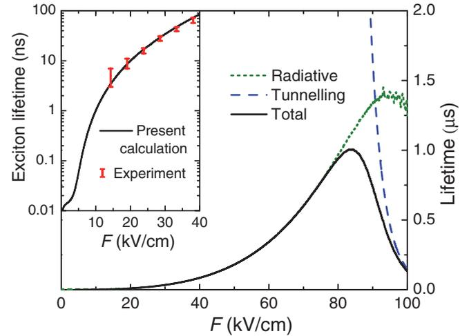
FIG. 10. (Color online) Radiative (dotted curve), tunneling (dashed curve), and total lifetimes (solid curve) of the exciton ground state X-GS as functions of the applied electric field. (Inset) Logarithmic plot of the X-GS total lifetime in comparison with measured photoluminescence decay times (error bars) extracted from Ref. 30.
