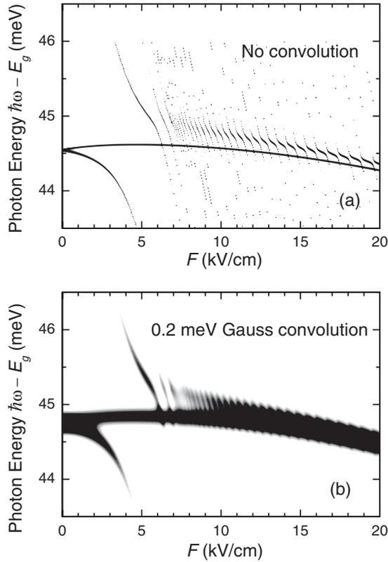
FIG. 11. (a) Electric field dependence of the full excitonic absorption spectrum. (b) The same spectra convoluted with a Gaussian function with 0.2-meV full width at half maximum.
