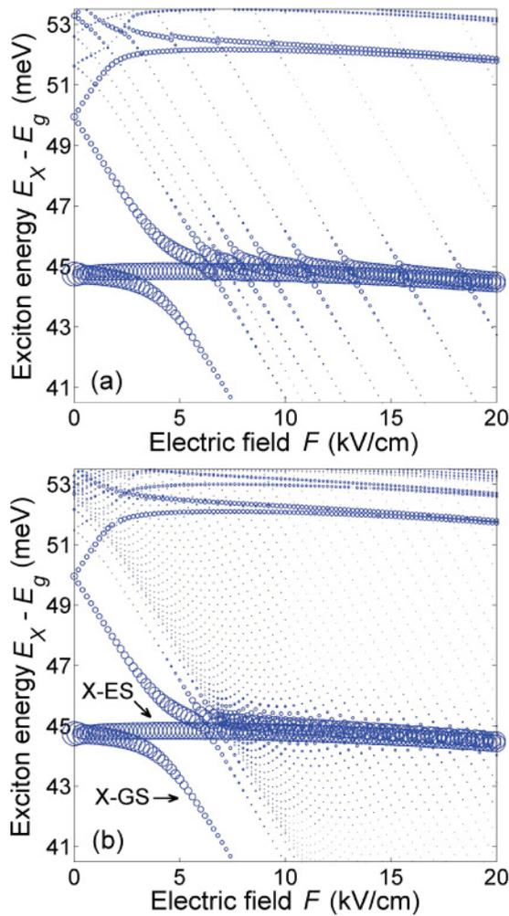
FIG. 4. (Color online) Electric field dependence of the optical transition energy  $E_X$  for different exciton states in a 8-4-8-nm GaAs/Al<sub>0.33</sub>Ga<sub>0.67</sub>As symmetric CQW structure, calculated using the exciton confinement radius  $R = 200$  nm (a) and 800 nm (b). The circle area is proportional to the exciton oscillator strength  $f$ .
