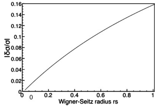
FIG. 1. Fractional change in the conductivity |\delta\sigma_{xx}^{ee}/\sigma_{xx}^0| for 0 \leq r_s \leq 1 . The current generation of topological insulators has r_s \ll 1 , so the theory presented in this work is applicable to these materials.
