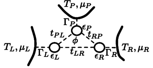
FIG. 2. Schematic drawing of the three-dot model.
