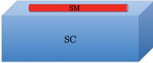
FIG. 1. (Color online) A semiconductor nanowire in contact with a bulk 3D superconductor.
