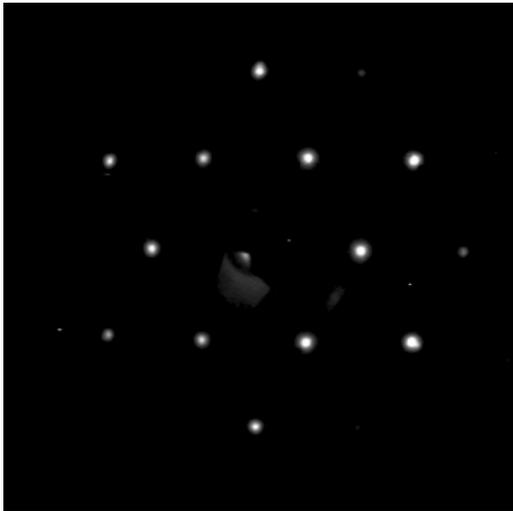
FIG. 1. LEED image of the  $\text{Mn}_5\text{Ge}_3$  surface. The sample temperature was 100 K and the primary energy of the electrons was 46 eV. The intense  $\sqrt{3}$ -diffraction spots are clearly seen.
