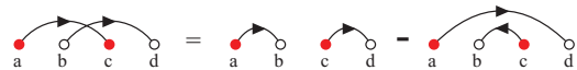
FIG. 19. (Color online) Illustration of the equivalence Eq. (A5), due to overcompleteness, between a state formed by two nonbipartite valence bonds and a superposition of two states involving only bipartite bonds.
