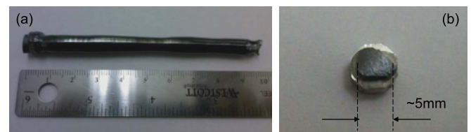
FIG. 2. (Color) (a) A whole volume of the \text{Mn}_3\text{O}_4 crystal grown using the floating zone technique. (b) Sample with surface normal along the [110] direction.
