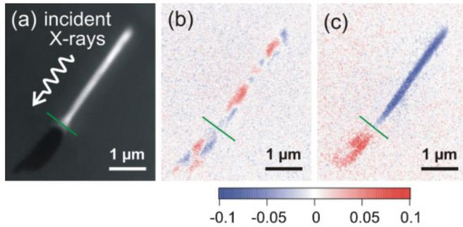
FIG. 4. (Color) (a) PEEM image of the core-shell wire taken at an angle of  $0^\circ$  between wire axis and incident x rays. (b) Differential XMCD image recorded at the iron  $L_3$  edge in zero magnetic field after annealing (as-prepared) and (c) after the first field sweep  $120 \text{ mT} \rightarrow -120 \text{ mT} \rightarrow 0 \text{ mT}$ . The blue and red XMCD contrasts represent magnetizations along and antiparallel to the wire axis, respectively. The green lines mark the wire end.
