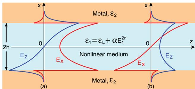
FIG. 1. (Color online) Schematic dependence of the electric field components  $E_x$  and  $E_z$  on the transverse coordinate  $x$  for (a) symmetric and (b) antisymmetric SPP modes of a nonlinear plasmonic waveguide, formed by a nonlinear dielectric layer of thickness  $2h$  and permittivity  $\varepsilon_1$  sandwiched between two metallic layers of permittivity  $\varepsilon_2$ .
