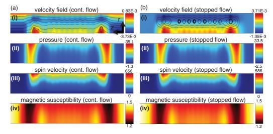
FIG. 5. (Color online) Simulated ferrohydrodynamic flow parameters at an input excitation of 9 A peak-to-peak, 1 kHz current excitation, both for continuous flow (a) and stopped flow (b) cases. The parameters include: (i) velocity field (unit: m/s); (ii) pressure (unit: Pascal); (iii) spin velocity (unit: rad/s); and (iv) local magnetic susceptibility (unitless) magnitude.
