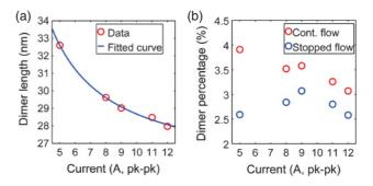
FIG. 4. (Color online) Field-induced dimer formation within the ferrofluid. (a) Effective hydrodynamic diameter of dimers as a function of the applied current amplitude, for both continuous and stopped flow. (b) Volumetric fraction of dimers among the total solid content within the ferrofluid, as a function of the applied current amplitude.
