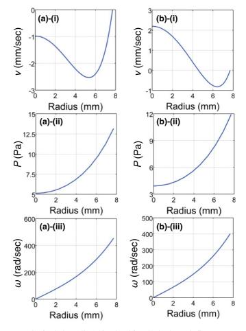
FIG. 6. (Color online) Simulated ferrohydrodynamic flow parameters at 9 A peak-to-peak current amplitude and 1 kHz frequency, both for continuous flow (a) and stopped flow (b), across the center of the pumping region (z = 0). The flow profiles include: (i) axial fluid velocity; (ii) pressure; and (iii) spin velocity.
