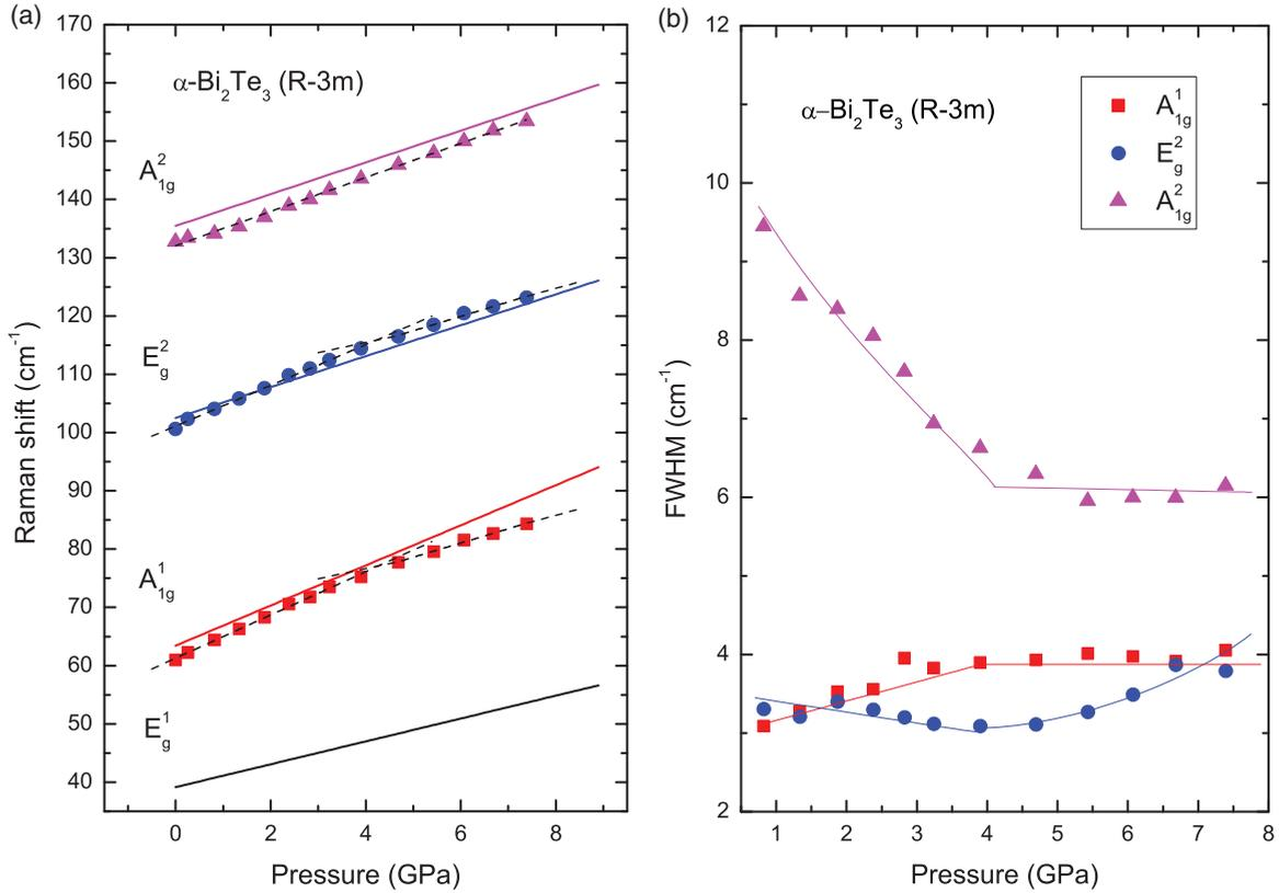
FIG. 6. (Color online) (a) Experimental pressure dependence of the Raman mode frequencies in  $\alpha$ - $\text{Bi}_2\text{Te}_3$ . Solid curves represent *ab initio* calculated-mode frequencies. Dashed lines are guides to the eye to indicate the different behavior of the experimental Raman mode frequencies with pressure. (b) Experimental pressure dependence of the FWHM of the Raman modes. Solid lines are guide to the eye to indicate the different behavior of the FWHM with pressure.
