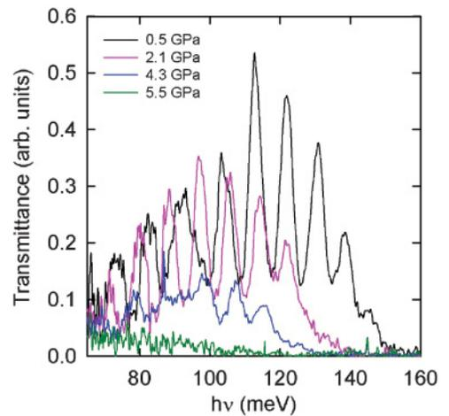
FIG. 2. (Color online) Experimental transmittance of  $\alpha\text{-Bi}_2\text{Te}_3$  at different pressures up to 5.5 GPa. A shift of the absorption edge to low energies is observed with increasing pressure.
