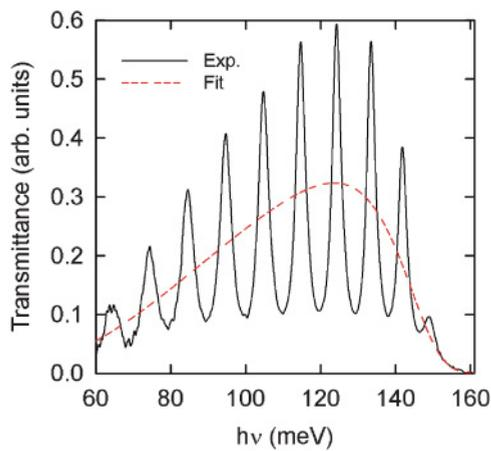
FIG. 1. (Color online) Experimental transmittance of a  $7\text{-}\mu\text{m}$ -thick  $\alpha\text{-Bi}_2\text{Te}_3$  sample at room pressure outside the DAC (solid line). Dotted line indicates the fit of the experimental spectrum.
