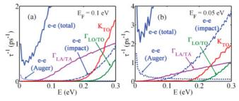
FIG. 3. (Color online) Simulation results for  $\tau^{-1}$  vs E (conduction band,  $\kappa = 10$ ) under equilibrium with (a)  $E_F = 0.1$  eV and (b)  $E_F = 0.05$  eV. Coulomb scattering rates are much larger than e-ph scattering rates and increase with decreasing  $E_F$ .
