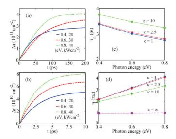
FIG. 4. (Color online) Simulation results for  $\Delta n$  vs *t* with optical pumping ( $E_{opt} = 0.4, 0.6, \text{ and } 0.8 \text{ eV}, P_{opt} = 20, 30, \text{ and } 40 \text{ kW cm}^{-2}$ ) for  $E_F = 0$  eV with (a) e-ph scattering only and (b) e-e scattering considered with  $\kappa = 2.5$ . (c) Relaxation time vs  $E_{opt}$  and (d) absorption efficiency vs  $E_{opt}$  for various  $\kappa$  values for the same optical pumping conditions.
