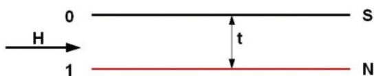
FIG. 2. (Color online) A superconducting (S)–normal metal (N) bilayer with in-plane magnetic field H .
